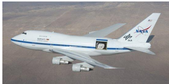
Fig. 13. SOFIA is a Boeing 747 SP modified to carry an open port 2.7 m telescope (chopped aperture 2.5 \text{ m} ), that enables routine access to the highest THz frequencies [84]
