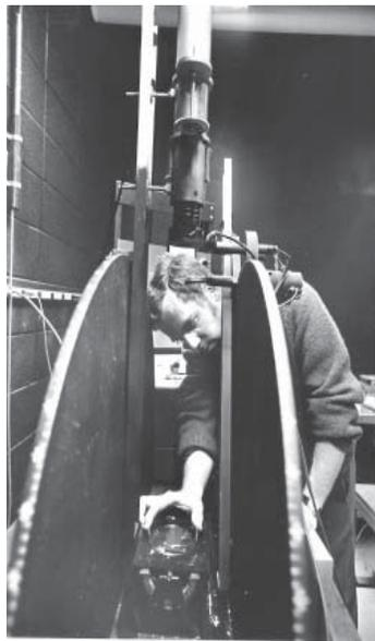
Above, Cornell astronomer Brian O'Leary preparing a lunar sample for analysis. Right, placing another one in the goniometer, an instrument used to determine the reflectivity of a sample as a function of the angle of the incident light. Photos: Cornell University.
