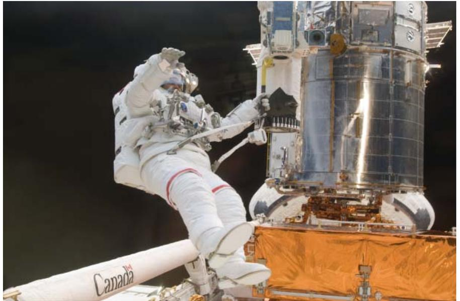
18 May 2009, eight day of flight and fifth day of repairs. Astronauts John Grunsfeld and Andrew Feustel (out of frame) installed a battery group replacement, removed and replaced a Fine Guidance Sensor and three thermal blankets (NOBL) protecting Hubble's electronics. Credit: NASA/Hubble Heritage Team (STScI/NASA).
