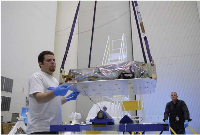
In the Payload Hazardous Servicing Facility at NASA's Kennedy Space Center in Florida, technicians attach straps from a crane in order to lift the Science Instrument Control and Data Handling Unit, or SIC&DH, which was installed by astronauts John Grunsfeld and Drew Feustel on the first day of repairs. Credit: *NASA/Jack Pfaller*.
