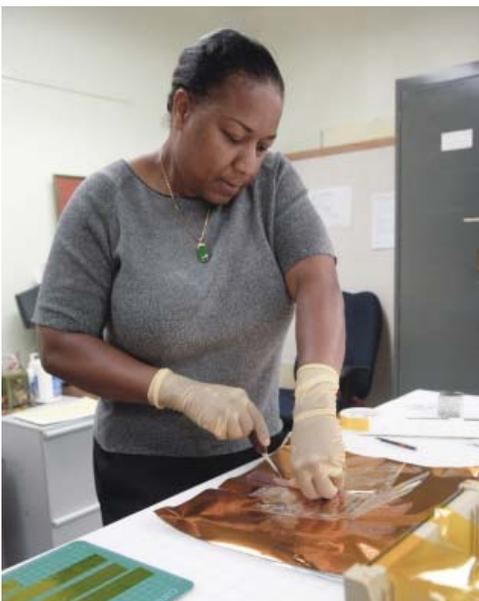
A technician cuts a piece of aluminum kapton film that became part of a thermal blanket. Credit: NASA.
