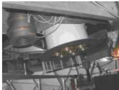
The 7-beam ALFA receiver installed in the Gregorian dome of the Arecibo telescope.
